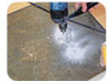
The first step in the ASTM F 2170 relative humidity test is drilling a hole to the proper depth of the concrete. Training in how to do moisture testing is offered in the IICRC (Institute of Inspection, Cleaning and Restoration Certification) Introduction to Substrate/Subfloor Inspection course. (Photo by Christopher Capobianco)
