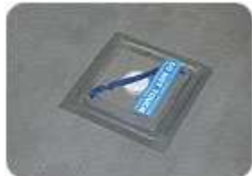
A properly placed calcium chloride kit: The building climate control system was operational, the floor was ground clean and left for 24 hours and the kit was placed. Adherence to the proper procedure is critical to accurate results.
