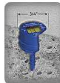
New technology in moisture testing makes it easier than ever to measure moisture below the surface of the concrete and make decisions about whether the concrete is ready to receive floor coverings. (Photo Courtesy of Wagner electronics)
