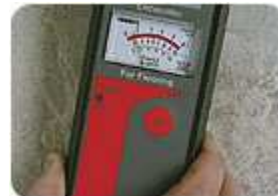
If it were only this easy...hand-held concrete moisture meters have their place but they are not to be used to decide if a concrete slab is ready for resilient flooring installation. (Photo Courtesy of Tramex)
