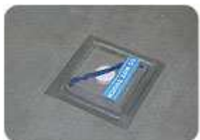
The Calcium Chloride Test (ASTM F 1869) is an accepted method for concrete moisture testing that has been in use for more than 50 years.
