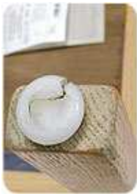
This broken chair glide was the culprit in a complaint for “cuts in the floor.”
