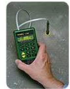
All concrete slabs must be tested for moisture regardless of how old they are. This photo shows the ASTM F 2170 "in Situ" Relative Humidity test that measures moisture inside the concrete slab. (Photo courtesy of Sean Fallon of Tramex)
