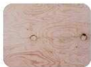
Plywood with knots should not be covered with resilient flooring or patched. An underlayment should be installed to provide a smooth substrate
