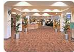
From Wicaders Cork Oak Flooring's WickCork Identity Collection, the flooring seen here is designed to withstand the heavy traffic of a commercial environment. It has been treated with the company's Xtreme Wear Resistance Technology which is created by laying a fine shield of ceramic micro-beads to protect and from scratches, scuff marks, abrasions, and even UV damage.
