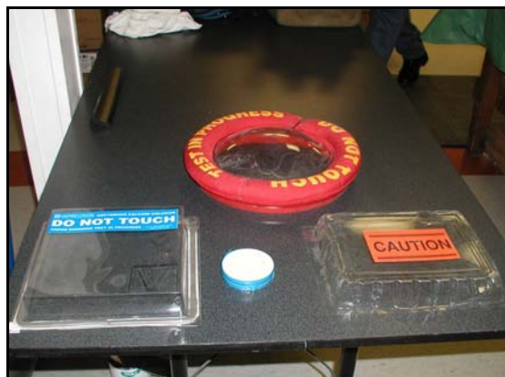
ASTM test F 2170 measures the internal relative humidity of a concrete slab.
