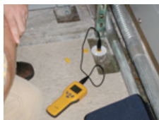
A relative humidity meter connected to the probe yields an internal moisture reading. Relative humidity testing represents advanced concrete moisture testing for the 21st century.
